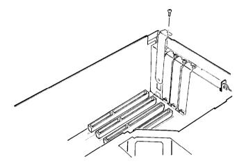
Keep the screw to secure the option card to the computer. Store the slot cover in a safe place in case you remove the option card later.
